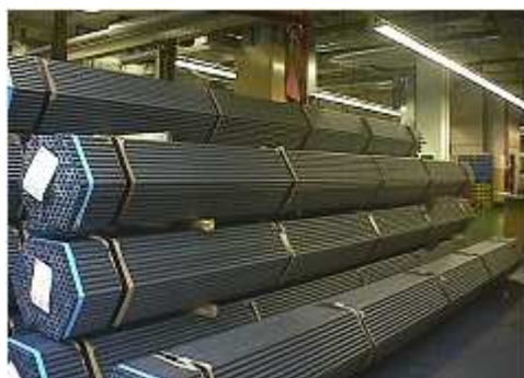
Figure 3: Packaging of tubes for overland transport
